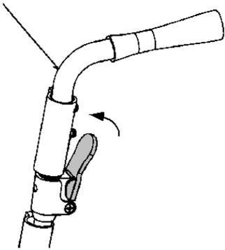
Push the black paddle (arrowed) towards the back post with your thumb whilst pulling the handle down. Repeat this operation for the other handle. To put the backrest back into position, lift both handles together and the folding mechanism will lock back automatically.
